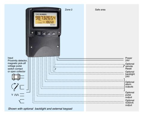
The BA334ND is an externally powered, Type nL certified rate totaliser with separate rate and total displays which will operate from a switch contact, voltage pulse, magnetic pick-off, open collector or a proximity detector input. A novel adaptive measuring technique plus an adjustable digital filter ensure that optimum rate display stability and step response can be achieved over a wide input frequency range.
